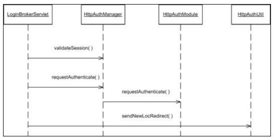
The login-broker servlet invokes the method validateSession() on a HttpAuthManager instance. The HttpAuthManager method validateSession() calls the doAuthenticate method on the module installed on the HttpAuthManager class. The servlet uses the boolean result of this method to determine whether to invoke the method sendNewLocRedirect() on the HttpAuthUtil class, or to trigger the requestAuthenticate() method on HttpAuthManager Object.
